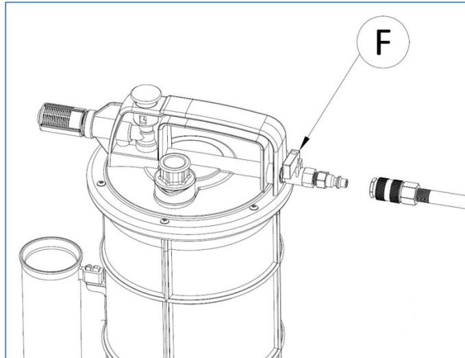
8. Turn Air Valve Switch (F) to the open position ( $\frac{1}{4}$  turn clockwise) and press the Push Button (E).
