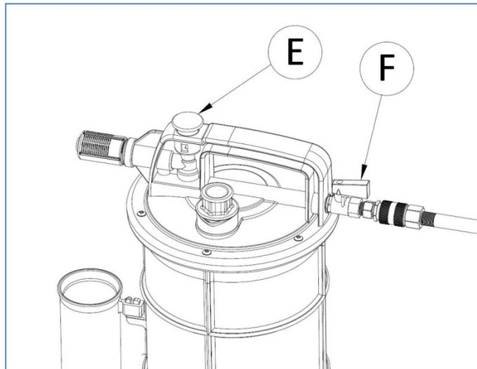
9. When the Reservoir Tank (J) is full, the extractor will automatically shut off. If extractor does not become completely full, turn Air Valve (F) to the off position in order to stop the extractor. Proceed to Step 12.
